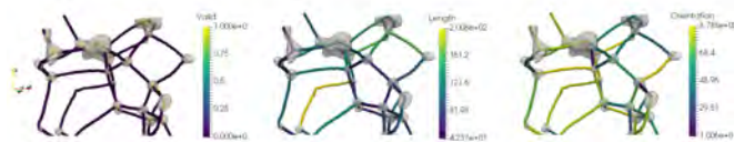
Fig. 15: Some of the metrics extracted for the ligaments. On the left, a binary field indicates when a point along the ligament is inside a junction or not, in the middle, the color of the tubes indicates the length of each ligament; and on the right, the color indicates the orientation respect to the Z axis of the ligament.
